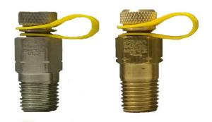
Pete's plug/ Test plug are time and money saving device which are used to check the pressure and temperature readings swiftly. It eliminates the need of permanent installation of costly pressure gauges or temperature indicators on the line. Pete's plug/ Test plug consists of two self closing valves that improves the speed of valve closure.
